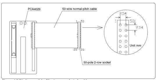
Figure 4.8 Pin layout of the 50-wire normal-pitch cable
